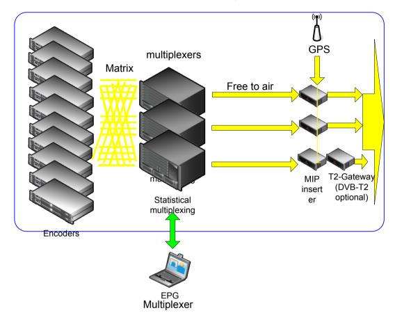
In order to guaranty the minimal allowable video quality no more than 8 SD streams per MUX are allowed in combination with MPEG 2.
