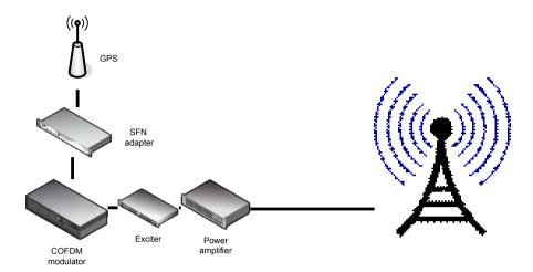
The transmitter setup consists of standardised DVB-T/T2 capable equipment wich features a dedicated GPS receiver for SFN operation.
